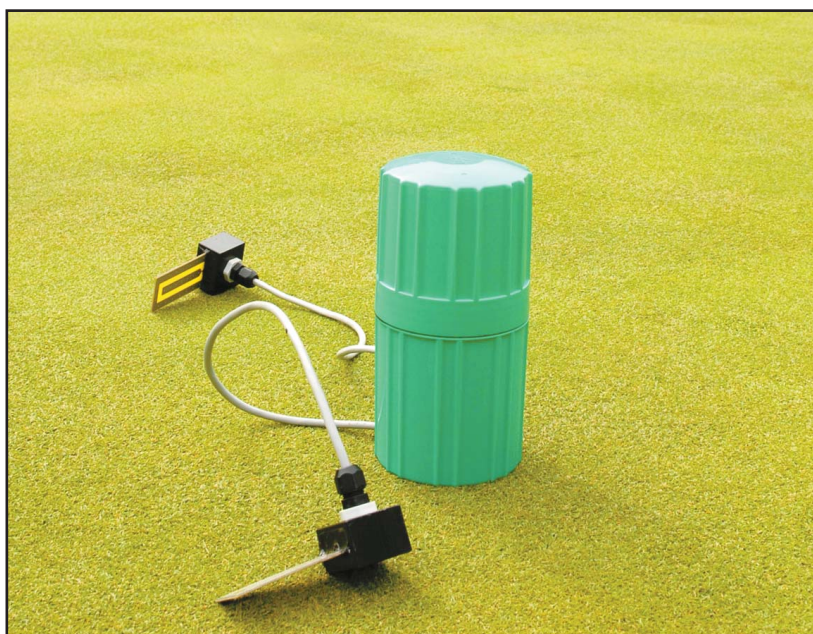
MCT photo The wireless transmitter and sensors of the UgMO soil monitoring system are installed on a green at the Merion Golf Club in Ardmore, Pa. Golf courses have embraced the technology, which Walter Norley says has the ability to achieve water savings of at least 25 percent.
